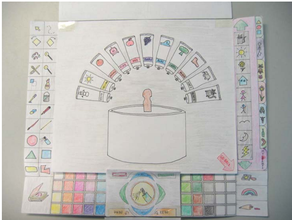
Figure 2 Interactive low-fidelity prototype with flaps that show changes in interface depending on tool or state.
